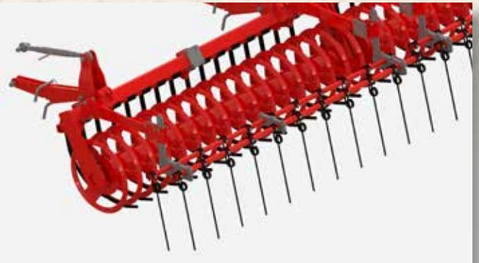
**2ST: 2-ROW TRAILED WEEDER TINES WITH Ø 10 mm / 0.39" INSTEAD OF CRUMBLER**
