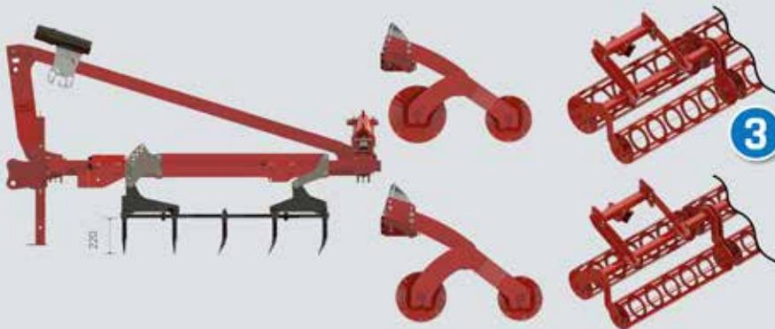
Section with arable harrow tines with flat rod- & serrated crumbler
