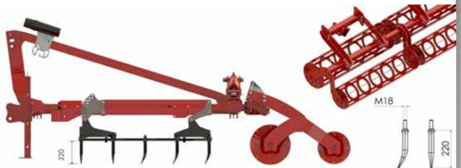
**G-2FZ: mini seedbed tine section + flat rod crumbler Ø 380 mm / 14.96" + serrated crumbler Ø 320 mm / 14.96"**
