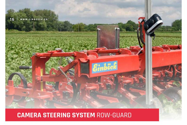
The ROW-GUARD camera steering system steers the hoe with absolute precision along the crops via a sideshift frame. This guarantees precise and close work of the hoe even at high speeds and will relieve the driver. Even with very small plants (from approx. 2 cm / 0.80") as well as in different colors or with heavy weeds, the ROW-GUARD camera steering in organic and conventional cultivation brings increased precision.
