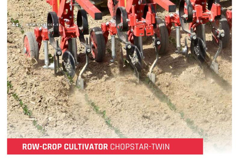
The CHOPSTAR-TWIN precision hoe was developed for precise hoeing above the row. The hoeing parallelogram does not work between the rows, but is mounted directly above the row. This allows a very narrow hoeing belt, which makes it possible to hoe young crops very early and narrow at the same time.
