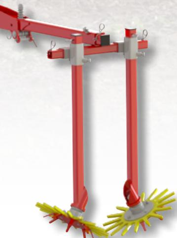
The finger weeders allow weeds to be pulled out and spilled between plants. They cannot be adjusted in angle to each other, as the fingers move parallel to the ground in the row of plants anyway when adjusted correctly. Finger hoes are also available for front machines
