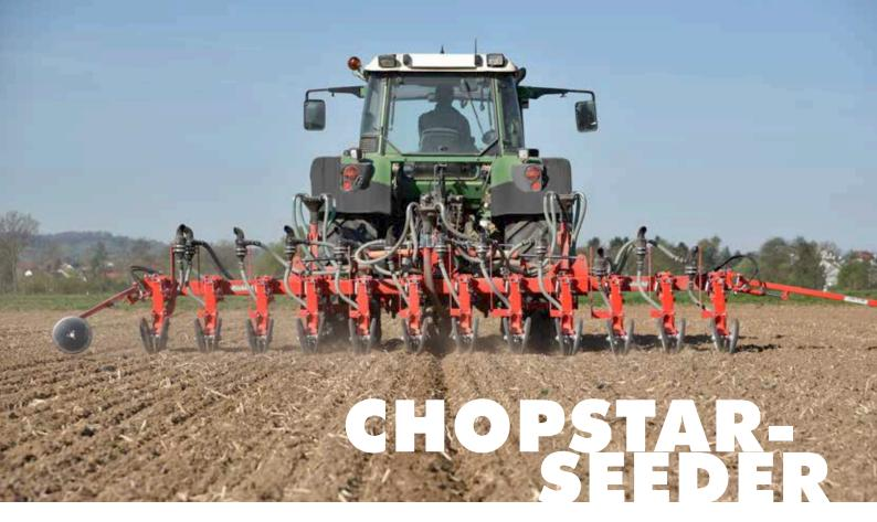
The CHOPSTAR-SEEDER ist flexible to use, because without any problems you can mount the hoe elements from the CHOPSTAR row crop cultivator program to the profile tube frame. So you get a wholesome row crop cultivator. Combined with the front tank you can use it additionally as fertilizer distributor.
