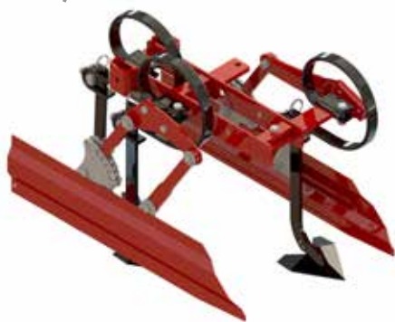
Hoe section CHOPSTAR 25-59 cm / 9.8-23.3", with hinged crop protection shields and vibrotines for shallow operation
