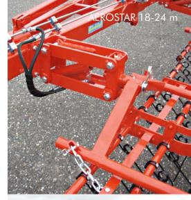
The suspended beam system by Einböck gives the tined weeder sections the same pressure independently from the position.
