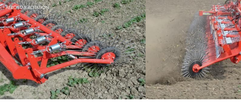
**6.5 mm / 0.26" thick spring steel tines**, cast into an inclined plastic disc do the job. Each of these 50 cm / 9.7" big star wheels is suspended separately, therefore they adapt perfectly to any surface irregularities.
