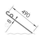
For **rocky soil** we recommend this straight tine so that the rocks are not moved to the surface. It has a diameter of 8 mm / 0.32" and a length of 490 mm / 13.9".
