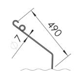
This standard universal tine with a diameter of 7 mm / 0.28" and a length of 490 mm / 19.3" is ideal for **medium to heavy soil conditions**. This tine length can also compensate uneven spots in the field.
