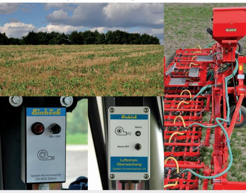
With **this control unit**, that can easily be mounted in the tractor cabin with a velcro, you can switch on/off the electric fan.
