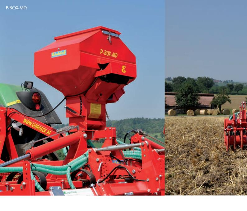
The flexible drive shaft flanged to the rubber support wheel or tail wheel transfers the power to an infinitely variable oil-immersed gearbox, which powers the seeding roller and the stirring shaft by a chain drive.
