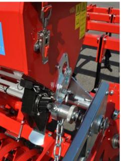
The DRILLBOX/MECHANICBOX is suitable for the use on rigid tilling implements. In a very easy and solid way you can seed 5 kg/ha of any intercrop seed and seed mix in a simple oversowing procedure using a knob for fine and a lever for coarse settings. The seedbox features an activation wheel system with baffle plates and can also be equipped with a stirring shaft for an extra charge.
