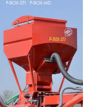
On request the airseeders are available with a **500 litres seed tank** (with tank support and extra-large opening).
