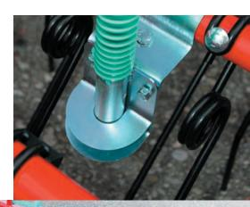
The standard P-BOX has 8 sections on the seeding roller, but with special rollers in combination with sealing plugs the outlets can be reduced. You can also use distributer heads for doubling the outlets (e.g. 16 outlets from eight sections).
