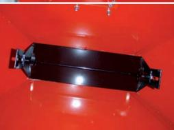
For heavy seeds we recommend the **retaining plate** mounted above the stirring shaft and the seeding roller.
