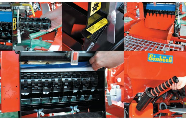
The **seeding roller** distributes the seeds into the eight divided and separated outlets. From there it is transported pneumatically via the PVC seed hoses to the deflector plates from where it is exactly spread over the entire working width. Since the seeds are blown pneumatically, wind does not matter as much as it would with mechanical seeders.
