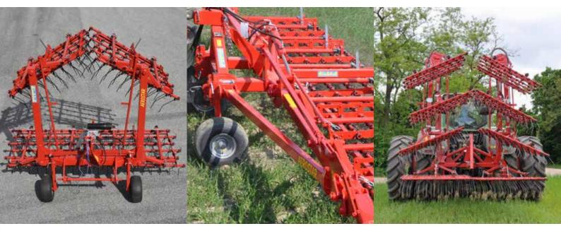
Folding the side sections will reduce the width of the AEROSTAR to a **transport width of only**2.6 m to 3 m / 8.5 ft to 9.8 ft.
