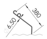
The tine with a diameter of 6.5 mm / 0.26" and a length of 380 mm / 15" is particularly suitable for **medium soil**.
