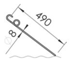
For **rocky soil** we recommend this straight tine so that the rocks are not moved to the surface. It has a diameter of 8 mm / 0.32" and a length of 490 mm / 13.9".
