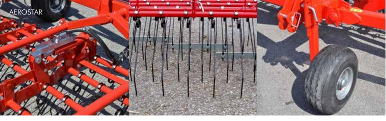
The hydraulic tine adjustment will make using the AEROSTAR in changing soil conditions a whole lot easier. It also puts the tines in a flat angle when the AEROSTAR is folded.
