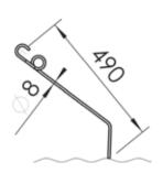
For **tough soil conditions** the tine with a diameter of 8 mm /0.32" and a length of 490 mm / 19.3" should be used. This tine is the most commonly used in grassland cultivation.
