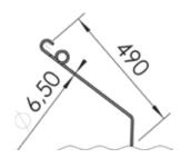
The tine with a diameter of 6.5 mm / 0.26" and a length of 490 mm / 19.3" is designed for **very light soil conditions.**
