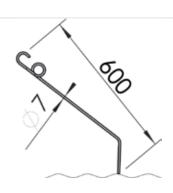
This tine with a diameter of 7 mm / 0.28" and a length of 600 mm / 23.6" is well suited for **special crops**. It also compensates for **uneven soil** very well. This is the least aggressive tine offered.
