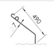
This standard universal tine with a diameter of 7 mm / 0.28" and a length of 490 mm / 19.3" is ideal for **medium to heavy soil conditions**. This tine length can also compensate uneven spots in the field.
